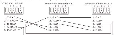
3、With multiple cameras connection diagram(PELCO-P/D)
