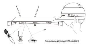
After the frequency of the transmitter and the receiver are synchronized, when speaking with the microphone, it indicates that the audio signal from the transmitter of this channel is received. When the transmitter and receiver are at the same frequency, this indicator will be on.
