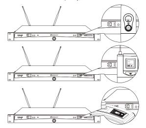
Channel display (the receiver and transmitter are at the same frequency)
