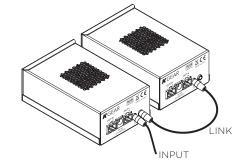
Prepare the speaker cable: set the 2.5/ 2-ST-5,08 euroblock plugs matching the loudspeaker polarity.
