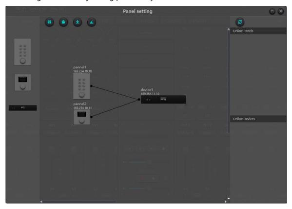
Offline device: It suits for offline edit status. Firstly, commissioning engineer configures panel parameters locally, and then download it to online panel. It is no doubt that the panel can be edited directly online. Drag offline device from the column of online panel to panel design area and then double click to edit it.
