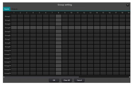
There are totally 16 groups. 1-device maximum number of channels can be selected for each group. the maximum number of channels is determined by the device type you purchased. Channels are set into one group which will be differentiated by a color in main interface.
