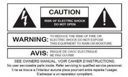
The lightning logo (an equilateral triangle with an arrow) is used to make the users aware of the uninsulated "dangerous voltage" within the product shell, which may cause electric shock. An equilateral triangle with an exclamation mark is adopted to make the users understand the importance of the operations and maintenance instructions given in the appendixes attached to the product.
