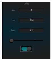
**Activate button**: Activate appointed delay module in modules and insert it into audio signal path to increase fixed delay time for signals.
