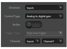
Analog-to-digital gain is very useful when connecting potentiometer externally. It may adjust input or output channel gain. It looks like rotary encoder. The difference between them is potentiometer analogs and adjusts voltage and current while encoder is digital and transmit the binary codes of 0 and 1.
