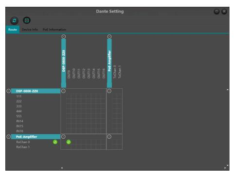
On the routing interface, the small boxes at the intersection of sending and receiving channels indicate that routing relationship can be created. Green icon will appear at the intersection of matrix after single click. Users may see a grey icon for a very short time period at the very beginning, which indicates that routing is in process.
