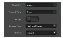
Trigger types: high level trigger/low level trigger/high level trigger, low level cancellation/low level trigger, high level cancellation, i.e., rising edge/falling edge trigger/rising edge trigger, falling edge cancellation/falling edge trigger, rising edge cancellation
