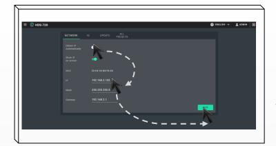
Turn off "Obtain IP Automatically", need to set the static IP address manually.
