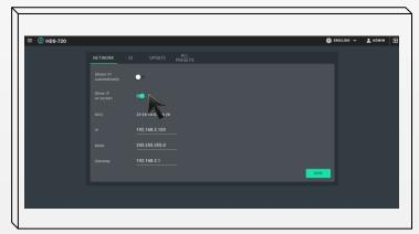
Turn on/off show IP on screen to enable/unable to see the IP in HDMI output.
