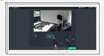
Controlling the camera by Up, Down, Left, Right, Zoom. Also choose the microphone ID to do the setting.
