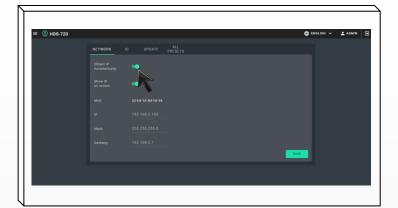
To set the DHCP function, check "Obtain IP Automatically"
