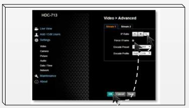
Set the IP Ratio to 10, check "Force Frame", click OK to save the setting.
