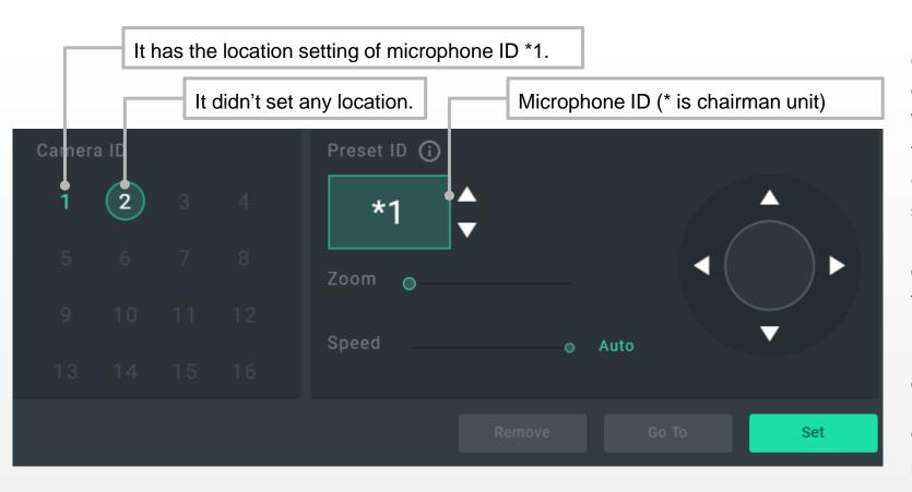
Camera ID's color also able to check the status of each camera. White "2": It's online status. Able to control and set the camera. Green "2": It has the location setting of selected Preset ID. Red"2": It's offline, unable to control and set the camera tracking.
