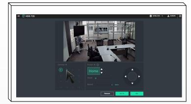
Choose the camera ID to control the camera and set the preset ID location.
