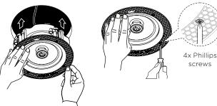
Reposition the grill on the loudspeaker.
